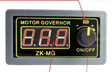
LED displays motor adjusting duty
